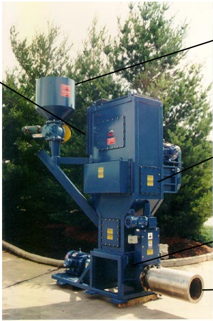
Hazardous Waste Shred/Feed System with water cooled extrusion tube, bulk and contaminated air lock in-feed.
