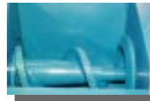
Feeder with continuous, variable feed rate producing air-sealed plug.
