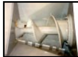
Easy to maintain screw auger
