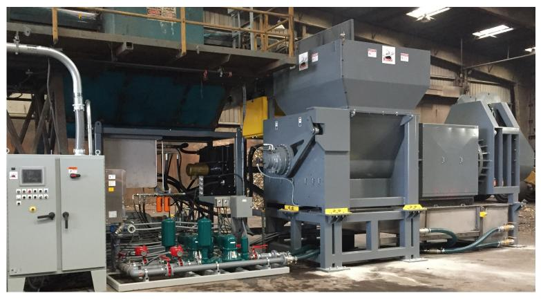
Athens Services has collaborated with Komar Industries to produce an Organic Separation Press (OSP). The machine combines a compression auger with a dewatering unit to separate nutrient-rich organics from municipal waste streams. The OSP processes about 40 tons of waste per hour. Of that, the machine is able to recover up to 40 percent for beneficial reuse.
