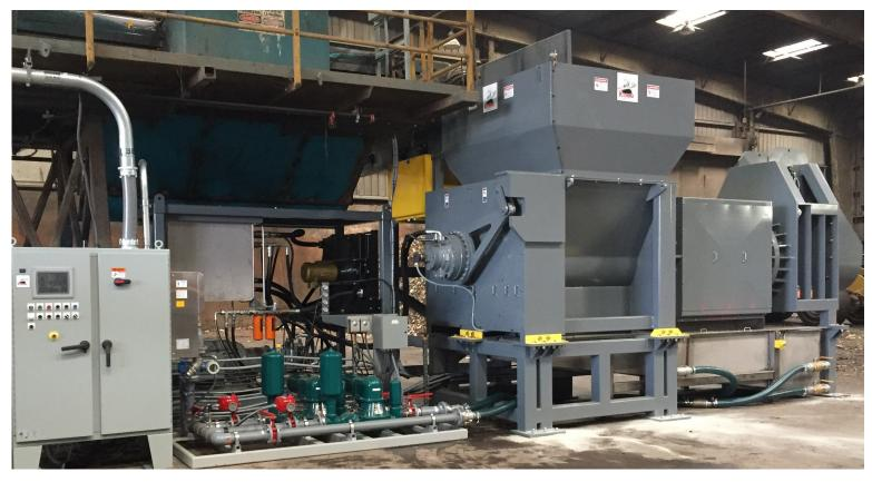
Athens Services has collaborated with Komar Industries to produce an Organic Screw Press (OSP). The machine combines a compression auger with a dewatering unit to separate nutrient-rich organics from municipal waste streams. The OSP processes about 40 tons of waste per hour. Of that, the machine is able to recover up to 40 percent for beneficial reuse.
