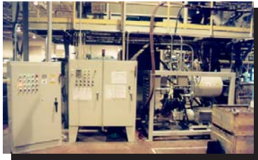
Independent machine control systems with pushbutton or touchscreen operator interface.
