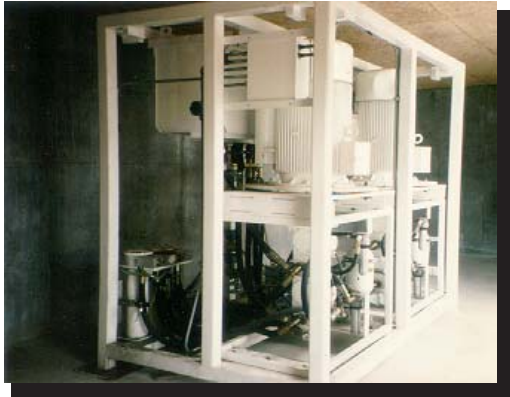
Power Units from 1 to 250 GPM - 1/2 to 400 H.P. single and tandem stacked variable displacement closed loop systems
