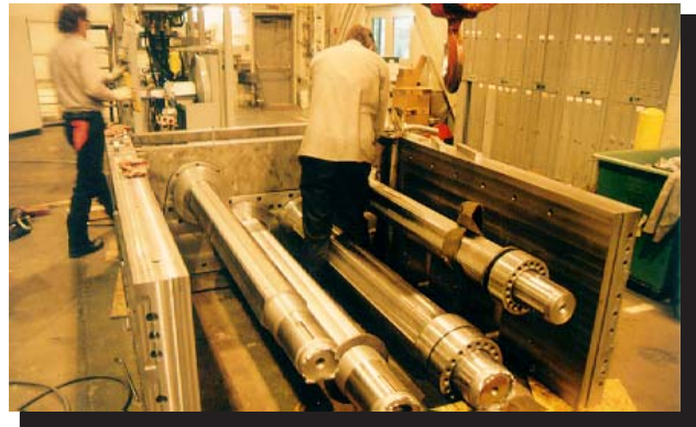
Four shaft shredder head assembly with stack up of close tolerance intermeshing cutters.
