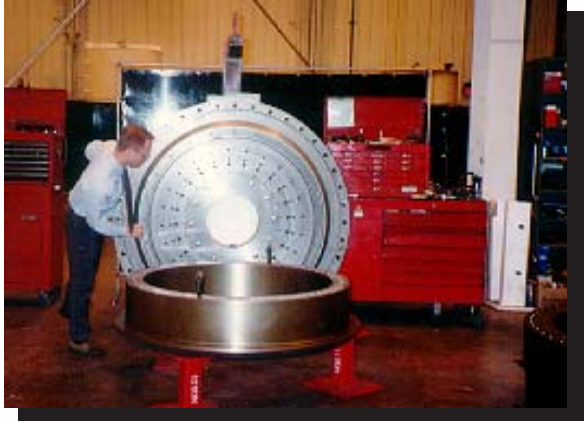
60" diameter bearing assembly completely assembled and tested.
