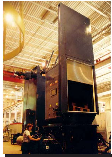
Complete assembly of incineration feed system for a pharmaceutical waste processing plant.
