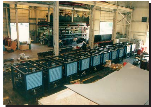
Production runs of Power Units - 200 H.P. closed loop displacement
